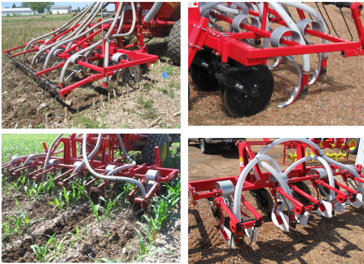
Figure 1. Injection equipment used for pre-plant application (top) and sidedress application (bottom) of liquid dairy manure.
